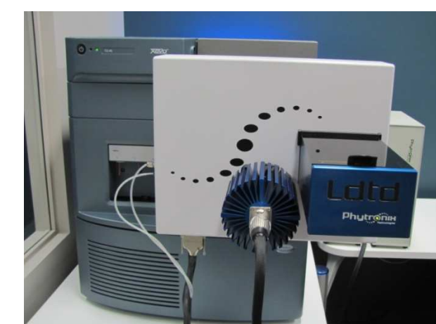
Figure 3 LDTD-MS/MS analytical system.
