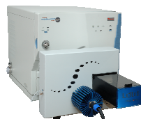
Figure 3 LDTD-MS/MS analytical system
