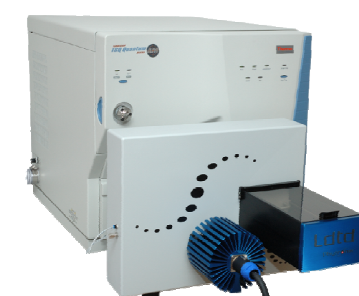
Figure 3 LDTD-MS/MS analytical system.
